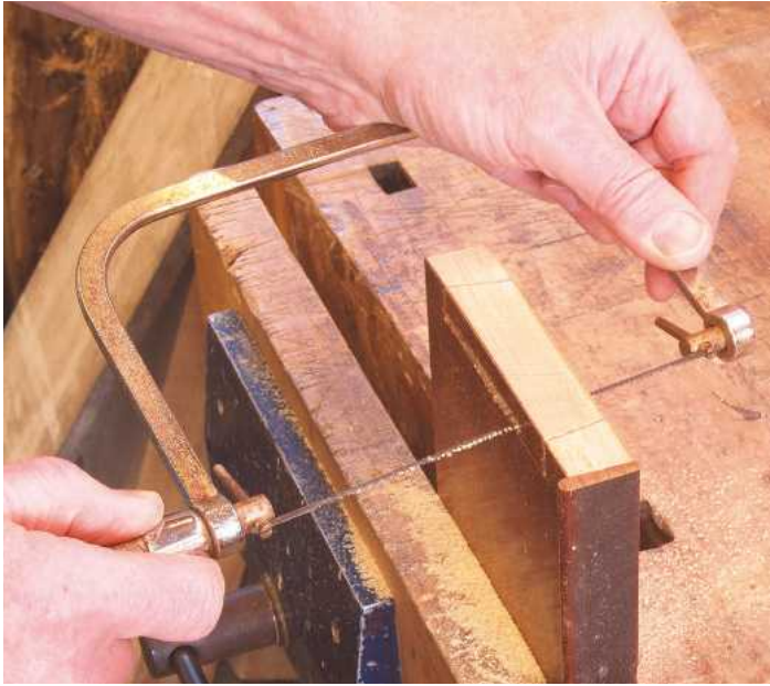
▲ Pic.10 Sawing waste with coping saw
